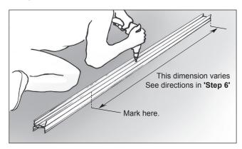
Step 6 - Mark the side of the posts with a crayon to set the finished height above the string-line. For example: For a 1.8 high fence on a level site, mark down from the top 1740mm (1720 +20 for the cap).
