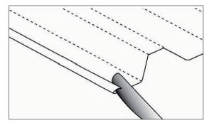
**Step 16** - Starting at one side slip the first Duopanel into the bottom rail (LH or RH panel). Ensure that the top of the Duopanel is between the stretchies.
