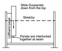
Step 18 - Repeat Step 17 with the remaining Duopanels, finishing with the LH or RH panel remaining (10 in all per 2.42 metre section).
