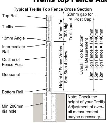
**Step 1 -** Assemble the frames and concrete into the ground as per standard fencing (bottom rail and top rail only).
