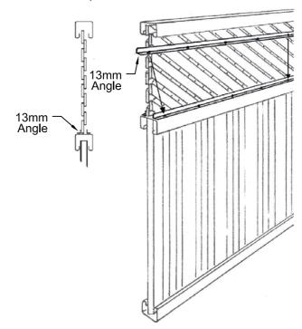
**Step 10 -** Before fixing the remaining tek screws, run a stringline along the middle rail to ensure correct alignment. Then fix all the remaining tek screws and fit the caps.
