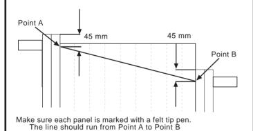
**Step 4 -** Dismantle the sloping panel and cut each individual duopanel with tin snips along the felt tip line.
