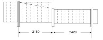
**Step 2 -** Insert all the duopanels as per Instruction Sheet A, bearing in mind that all full length panels have 10 duopanels, but the sloping panel will only have 9 duopanels (7 x standards, 1 x LH and 1 x RH). Support duopanels with the stretchies supplied.
