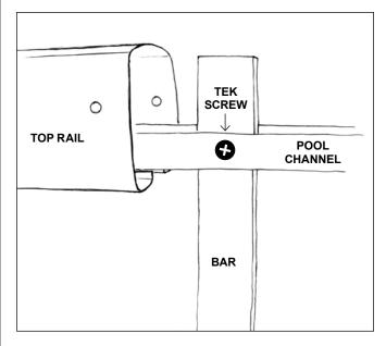
Step 11 - Slide the repaired infill back into the rail.
