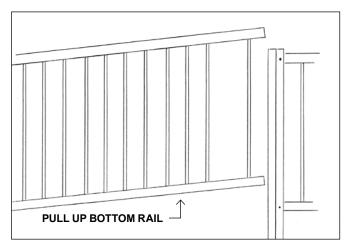
Step 5 - The bars and pool channel (with the square holes) can be slid out of the rails until you reach the hole that had the damaged bar.
