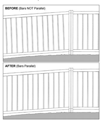
Step 2 - Tek screw through the top and bottom rail in line with the bar so that the tek screw pushes hard against the pool channel and the bar.
