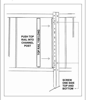
Step 4 - Tek screw the post to the rail insert on one side top and bottom.
